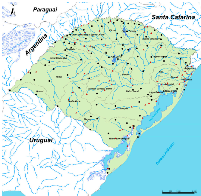
Map with the proposed location of 75 hydro meteorological gauges and plus 100 rain gauges to be installed in RS.
